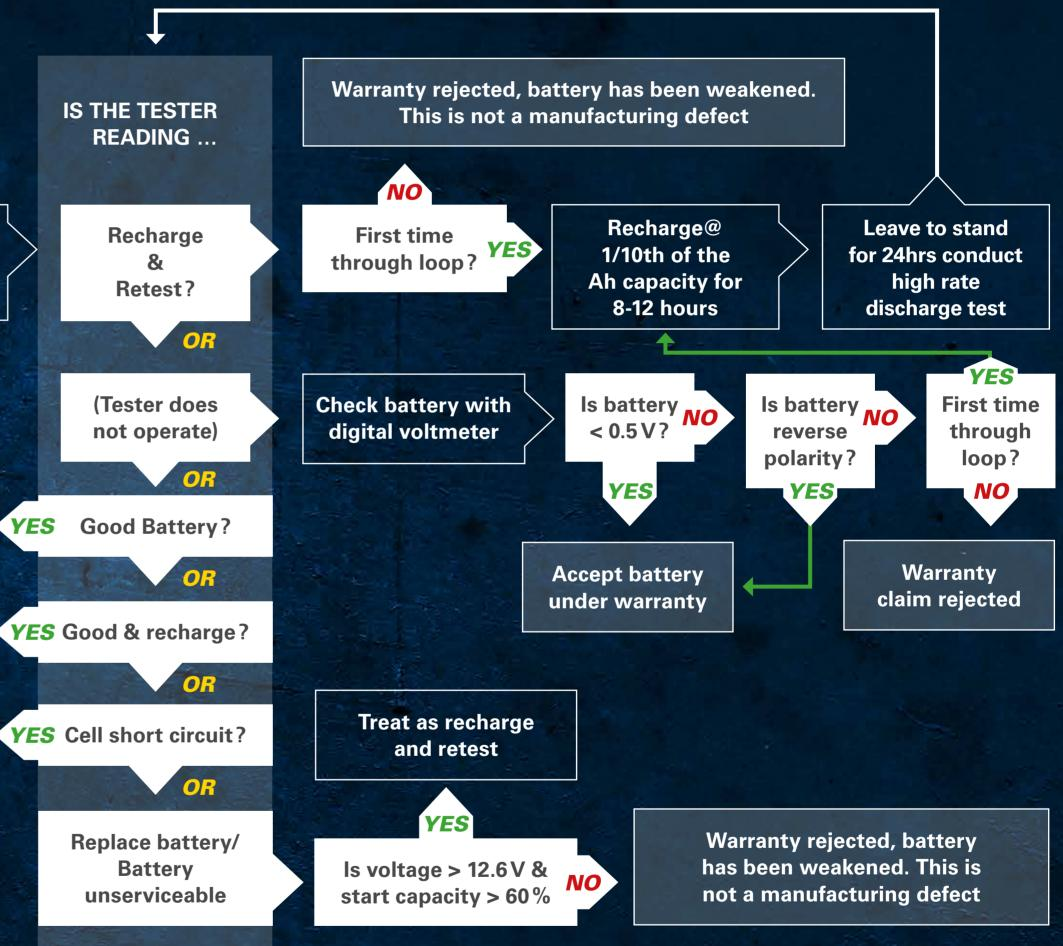
LOW TO TEST AND CHARGE A BATTERY
